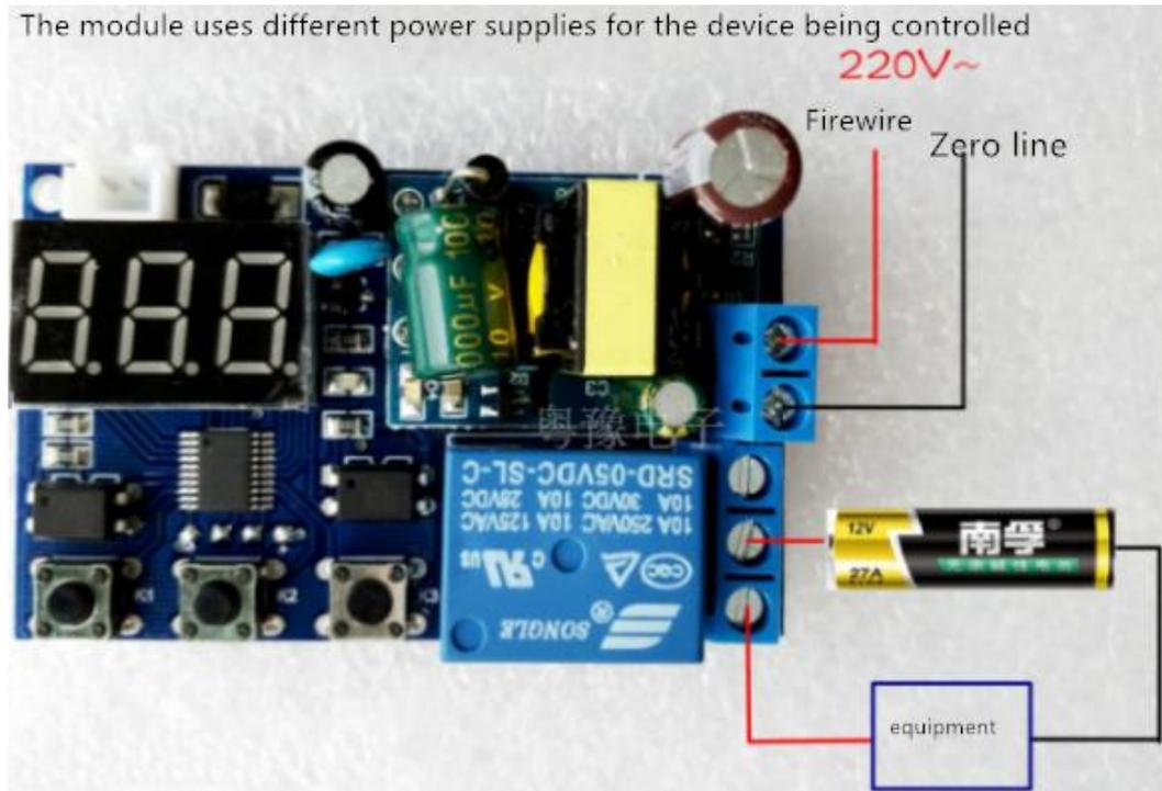
P-1: The signal triggers the relay to pull in, the time is up, the relay is off, during the delay:
