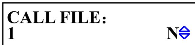
After entering Recall File page, file No. and file status are displayed in the second line. “Y” means the file has existed, and “N” means the file hasn’t been saved.
