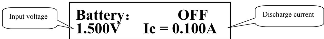
After the test, the following page is displayed. If time and capacity are not displayed currently, press **【ENT】** key to switch.
