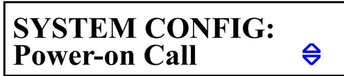
All the submenus in System Config can be selected through **【▲】** and **【▼】** keys or knob.
