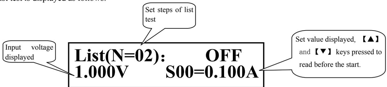
Related parameters should be set before list test starts. Press **【SHIFT】 + 【S\_LIST】** key to enter setting menu of list test. Refer to 3.4.5 for detailed information.
