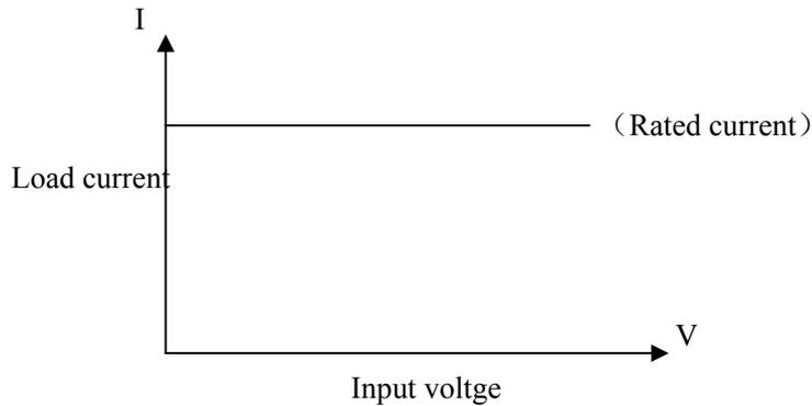
In other load modes, press **【I-SET】** key to enter constant current mode. Press **【ON/OFF】** key to start or stop working.
