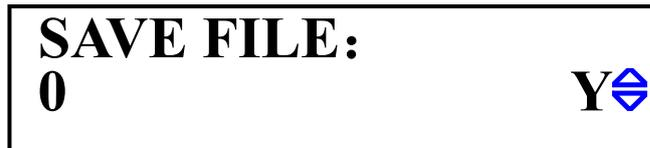
After entering Save File page, file No. and file status are displayed in the second line. “Y” means the file has existed, and “N” means the file hasn’t been saved.
