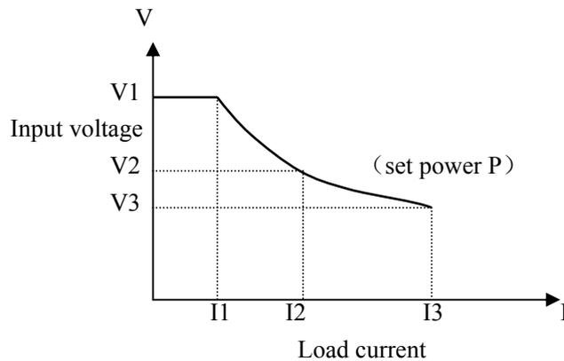
In other load modes, press **【P-SET】** key to enter constant power mode. Press **【ON/OFF】** key to start or stop working.
