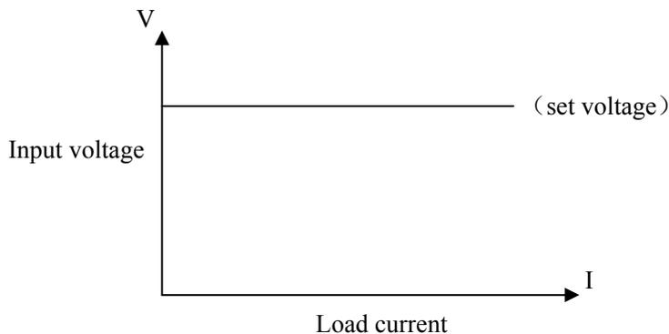
In other load modes, press **【V-SET】** key to enter constant voltage mode. Press **【ON/OFF】** key to start or stop working.
